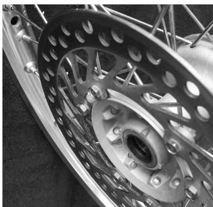
Left: Notice how the inner row of spokes on the far flange point clockwise, while the outer row points counter-clockwise. Also, see how their heads are recessed in the near side of this hub. Center: The partially installed spoke illustrates its specific features: The "head," "throat length" (distance it passes through the flange) and "angle" to match the direction to the rim. Right: The old wheel, half-way disassembled.
