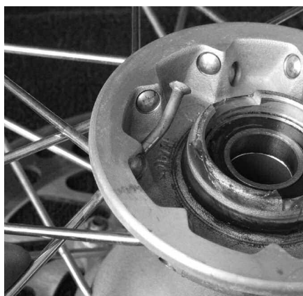
Left: Notice how the inner row of spokes on the far flange point clockwise, while the outer row points counter-clockwise. Also, see how their heads are recessed in the near side of this hub. Center: The partially installed spoke illustrates its specific features: The "head," "throat length" (distance it passes through the flange) and "angle" to match the direction to the rim. Right: The old wheel, half-way disassembled.
